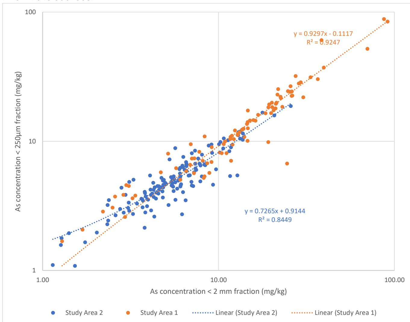
Figure 1: Comparison of arsenic concentration in the <2 mm and <250 µm size fractions includes both surface and subsurface soils with outliers removed. Note that the data are plotted on log-log axes.
