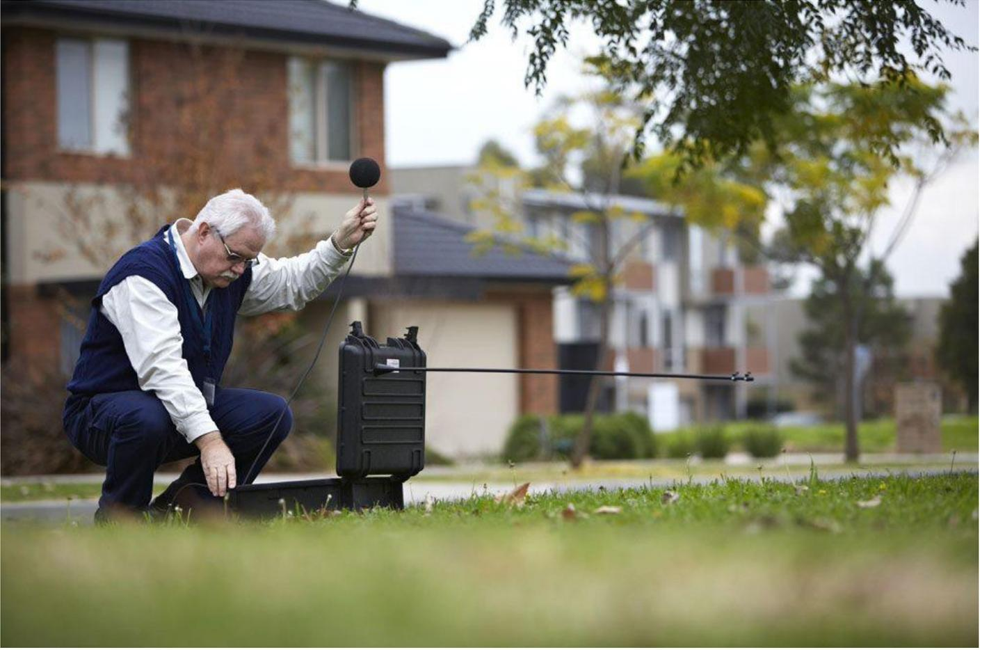
**Figure 11.** Noise emissions from concrete batching plants may be disruptive to surrounding residential communities. Noise monitoring can assist you to understand your compliance against regulatory noise limits. Source: EPA Victoria
