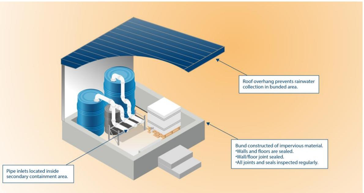
Figure 8: Effective volume of bundled area is 110 per cent of the volume of the largest container
